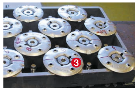
3 Markings to measure disc rotation
