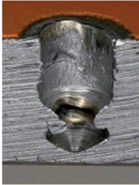
Steel base material after 10 years of exposure to sea water and pull-out of the X-BT fastener. The hole appears clean and no evidence of corrosion is visible.
