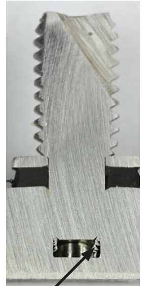
Displaced base material
